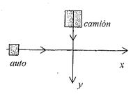
$$\overline{p}_{sist,,f} = \overline{p}_{sist,,i} \rightarrow (M_C + M_A) \overline{v}_f = M_C \overline{v}_{C,i} + M_A \overline{v}_{A,i}$$
